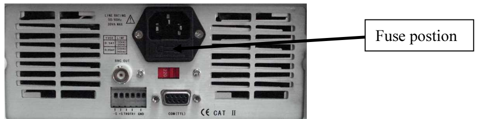
Picture 3.1 Fuse Location
